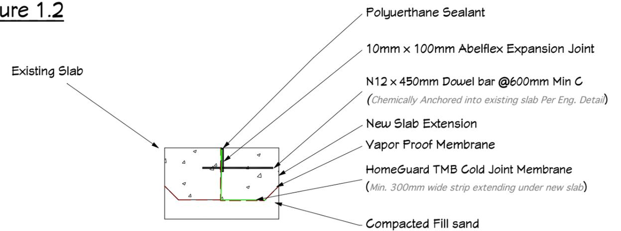
Existing slab to new slab intersection
