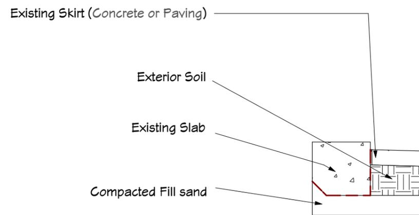
Existing Slab with Concrete or Paved Skirt to perimeter
